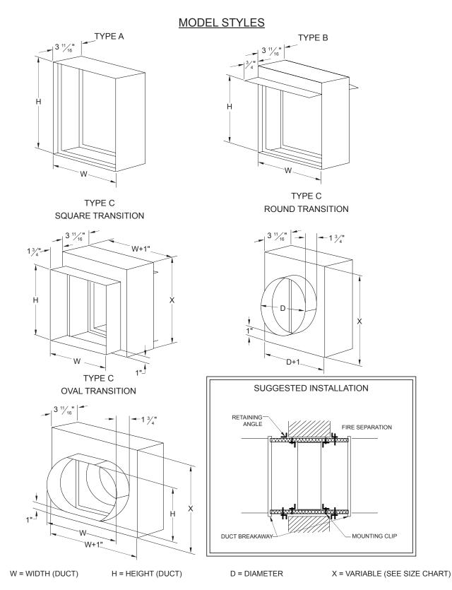
**NOTE:** Independent tests have shown a need for fire dampers in some HVAC systems to close against air flow. UL tests at present evaluate the performance and reliability of fire dampers under static and dynamic conditions. We recommend Metal-Fab, Inc. U.L. Classified dynamic closure fire dampers in HVAC systems that involve the possibility of fire dampers having to close against air flow.
