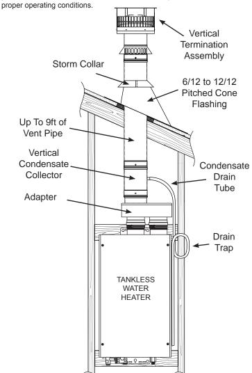
This kit can be extended up to a Maximum of nine (9) feet of vent pipe length DO NOT USE MORE THAT NINE (9) FEET OF ADDITIONAL VENT PIPING WITH THIS KIT. If more that nine (9) feet of vent pipe is used it could result in the improper operation of the tankless water heater. NOTICE: If a vent length of more that two (2) feet straight up from the top of the water heater is needed. a condensate collector must be installed at the water heater.
