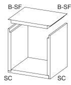
2-Piece "U" Duct and Closure Panel with (2) Foil Flaps
